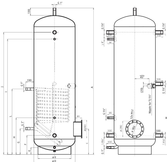
Socket G 1½" suitable for electrical heating element upon solar heating.
