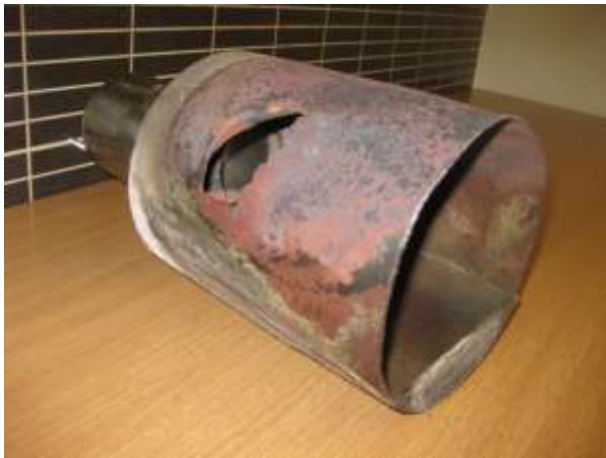
Photo 1 Burned-out burning chamber and deformed grate
