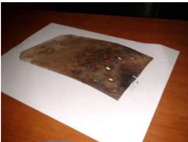
Photo 1 Deformed grate and burned-out burning chamber
