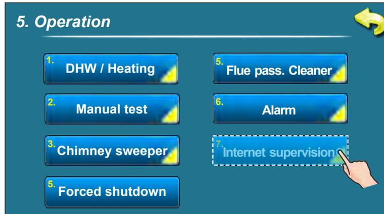
When "Cm WiFi box" is connected to the boiler and internet supervision is enabled, a new icon appears on the main screen showing the status of internet supervision.
