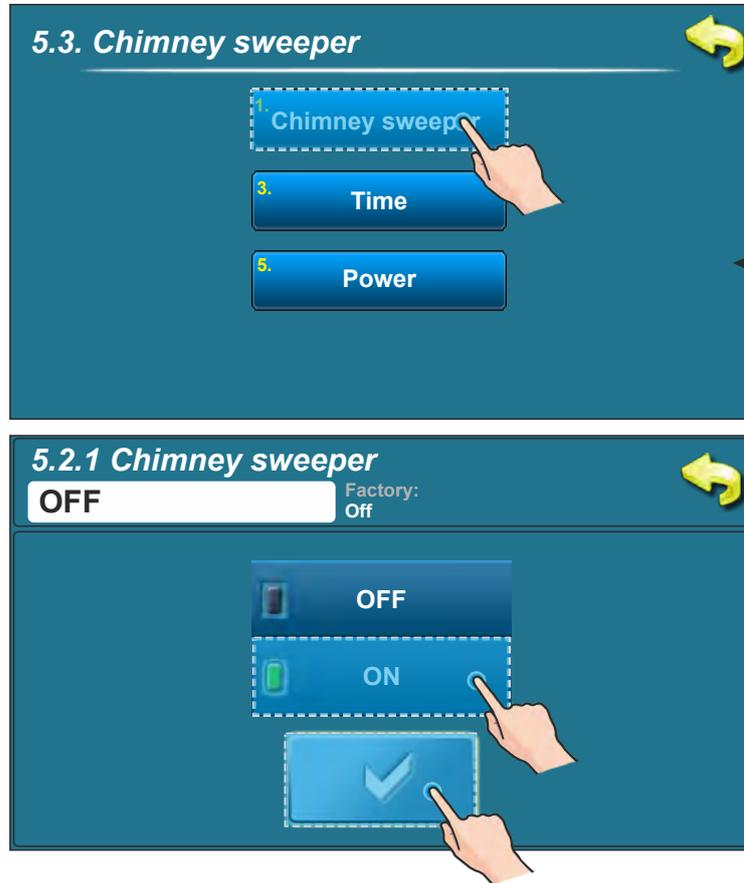
When this option is turned ON, button "BOILER OPERATION DISPLAY" becomes a button "CHIMNEY SWEEPER" (1). Pressing this button directly opens the menu "CHIMNEY SWEEPER" (without the need for scrolling through the menus). In this menu, is access to change parameters of "CHIMNEY SWEEPER" menu.
