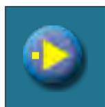
The pump has a request for work (next to the pump symbol bright yellow square when the consumer given the demand for work the pump, the pump does not work if you have not met all the conditions for work, for example. low temp. in the boiler, otherwise the pump normally works)
