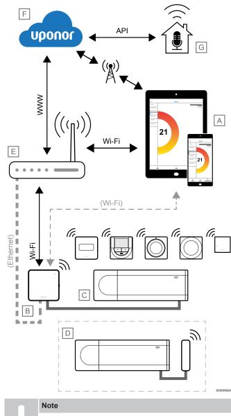
Setting up a system with a communication module requires a mobile device (smart phone/tablet).
