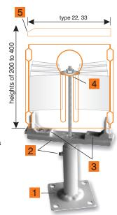
The "Plus" floor bracket is available in two different versions for finished floor surfaces (125 - 185mm) and for unfinished floor surfaces (185 - 285mm) and is suitable for heights of 200, 300, 350 and 400.
